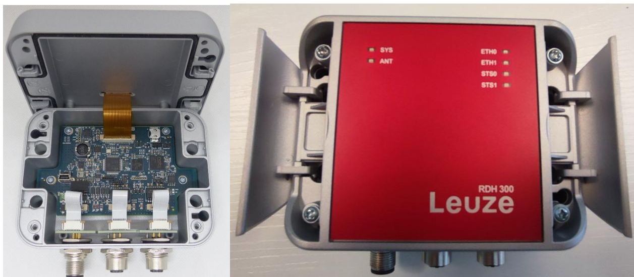
Figure 4: label to main board FPC connection and box cover screws.
